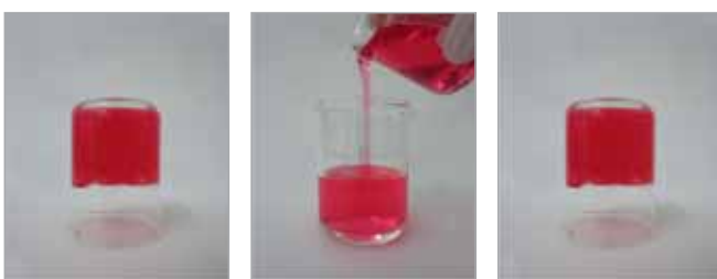
Room Temperature Heating Re-cooling LMA Pectin Gel
