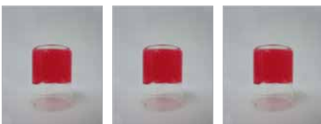
Room Temperature Heating Re-cooling LMC and HM gels
